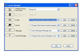
Launch Manager allows you to set the four easy-launch buttons located above the keyboard. **"Easy-launch buttons" on page 9** for the location of the easy-launch buttons.
